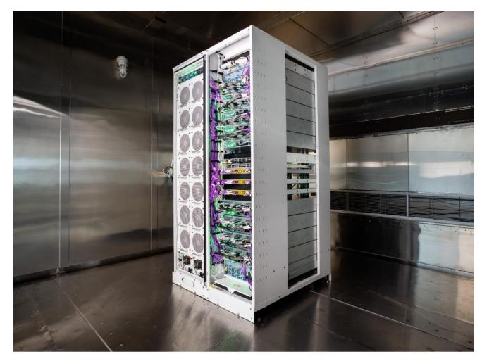
A custom-built rack for the Maia 100 AI Accelerator and its "sidekick" inside a thermal chamber at a Microsoft lab in Redmond, Washington. The sidekick acts like a car radiator, cycling liquid to and from the rack to cool the chips as they handle the computational demands of AI workloads. Photo by John Brecher for Microsoft.
